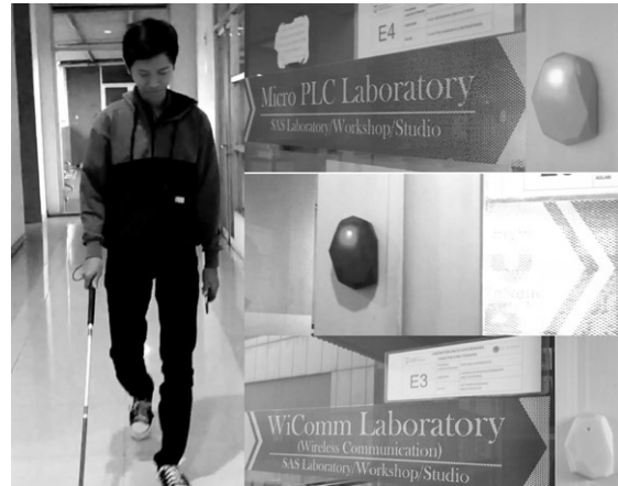
Figure 12: Estimote beacons Indoor Area Testing
