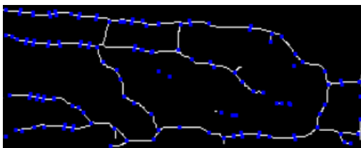
Figure 6: Corners extracted by Harris algorithm.
