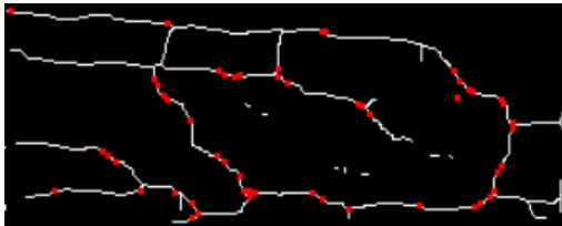
Figure 5: Corners extracted by FAST algorithm.
