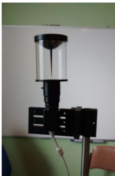
Figure 7: A catadioptric camera with an hyperbolic mirror.
