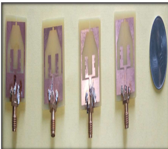
Fig 7: prototypes of proposed antennas with FR4 material.
