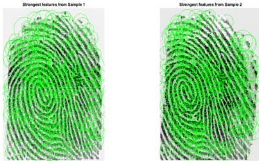
Figure 9 Detect and Select Strongest Points in Both Fingerprint Images
