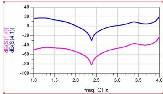
Figure 15: Simulation results of scattering parameters of coupler isolation
