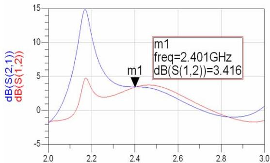
Figure 18: Tx and Rx gain simulation results.
