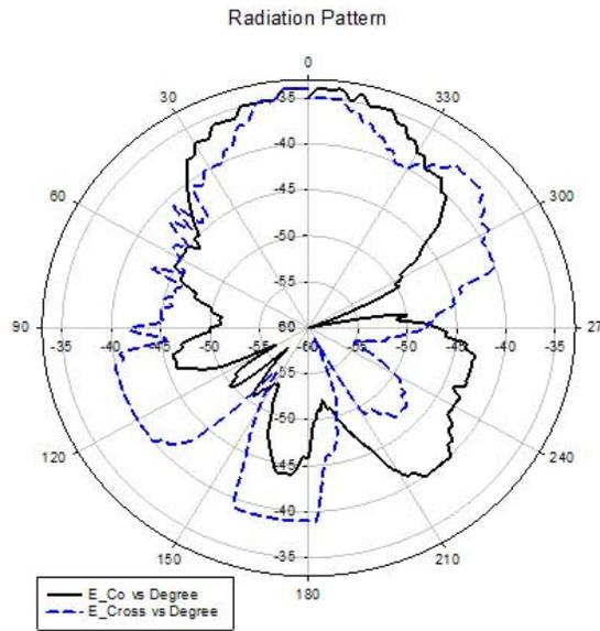
Figure 25. The E-plane of return loss in Active mode.
