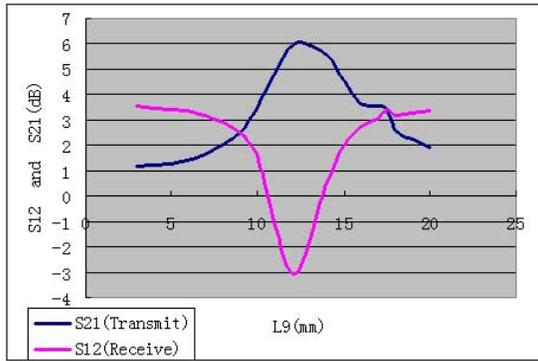
Figure 17: Adjustable L9 values to get the best gain the Rx and Tx channels.
