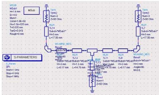
Figure 10: The schematic scheme of designed T-Junction produced by ADS software.
