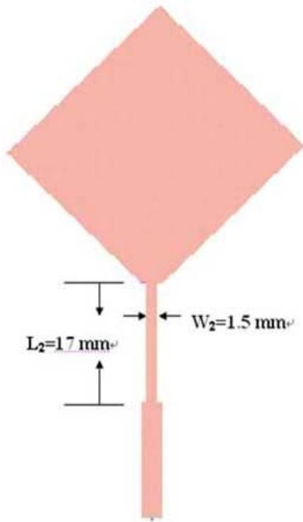
Figure 4: The Circular polarized antenna layout.
