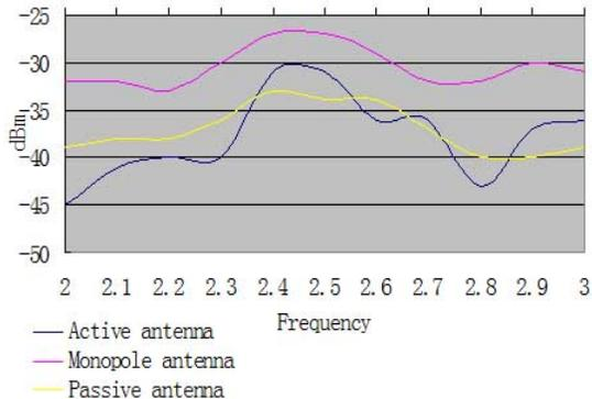
Figure 27: Comparing the gain of monopole antenna with the current active and passive antenna gain.
