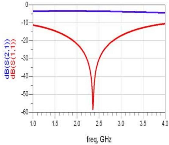
Figure 13: Scattering -parameters simulation results produced by ADS software for T-junction electronic power divider
