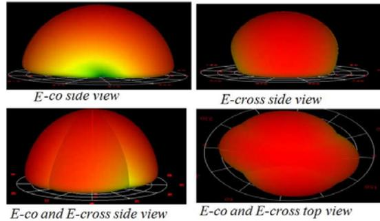
Figure 6: Elliptical polarization issued after simulated the radiation pattern of proposed square antenna.
