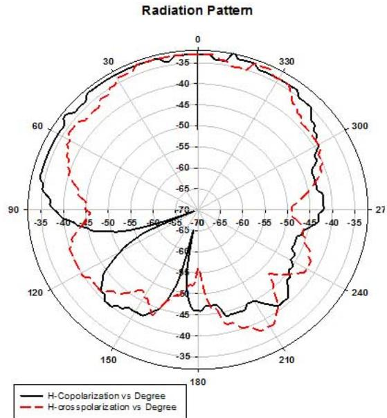
Figure 22: Radiation pattern of the Passive Antenna for H-copolarization.
