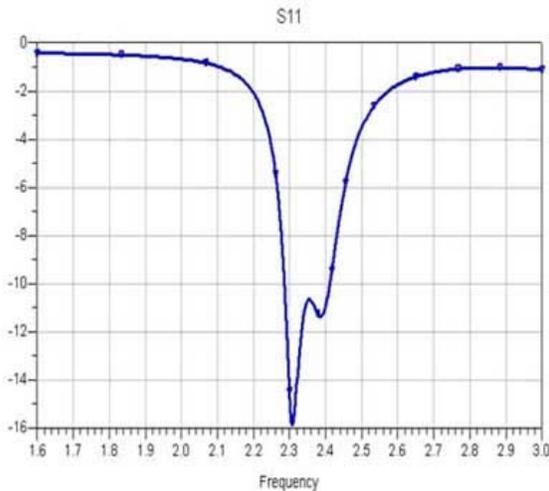
Figure 5: The return loss (S11) simulation results.
