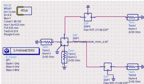
Figure 14: Coupler and amplifier combination of in ADS software
