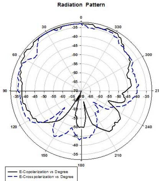
Figure 21: Radiation pattern of the Passive Antenna for E-copolarization
