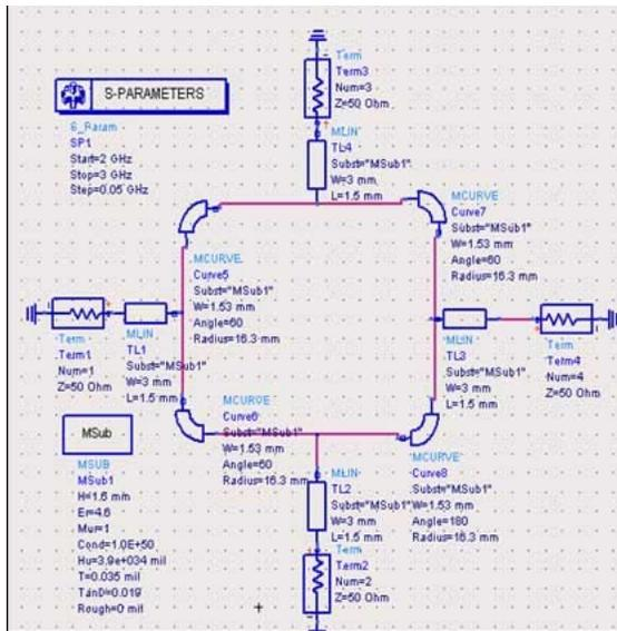
Figure 8 Schematic circuit mapping of Rat-race coupler.
