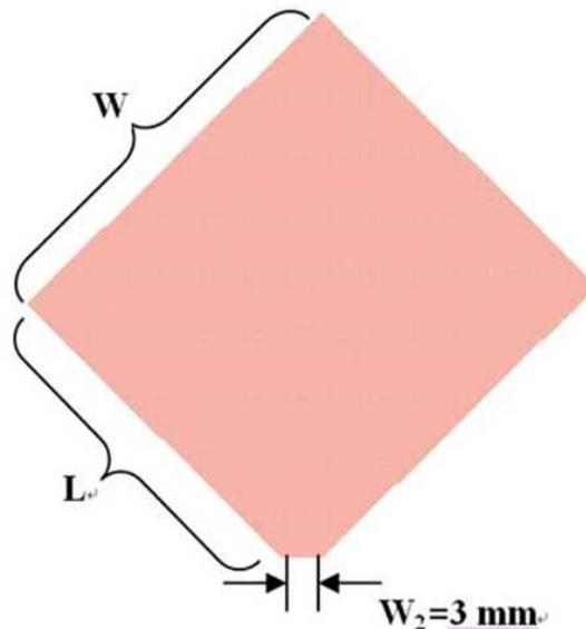
Figure 1: Microstrip antenna has a rectangular shape.
