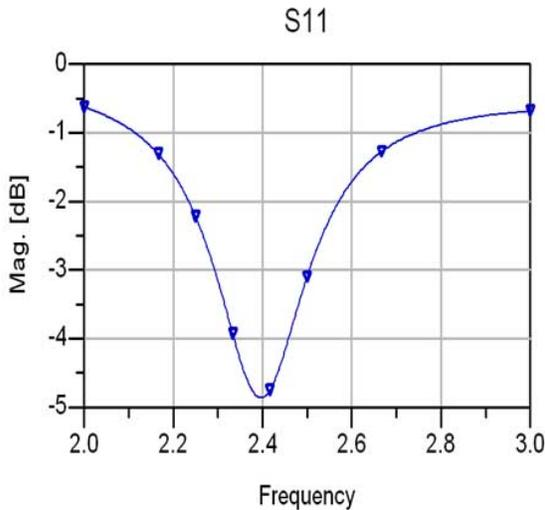
Figure 3:  $S_{11}$  simulation results for square antenna Layout
