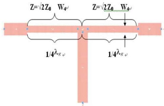
Figure 11: The Layout scheme of designed short T-Junction produced by ADS software.
