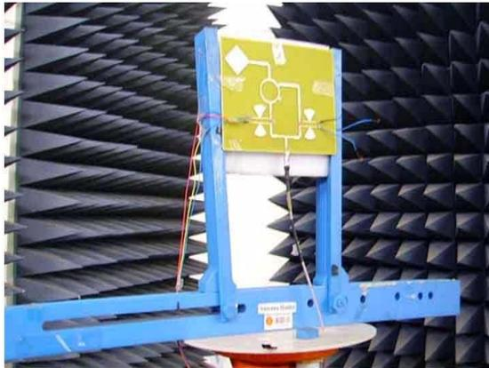
Figure 20: Measurement of antenna radiation pattern setup.
