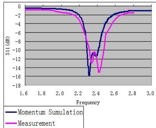
Figure 23: The measures Return loss in comparison with the simulated result.
