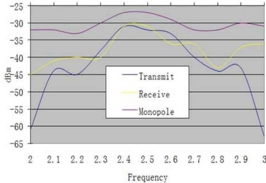
Figure 26: Comparing the gain of monopole antenna with the current active antenna gain.
