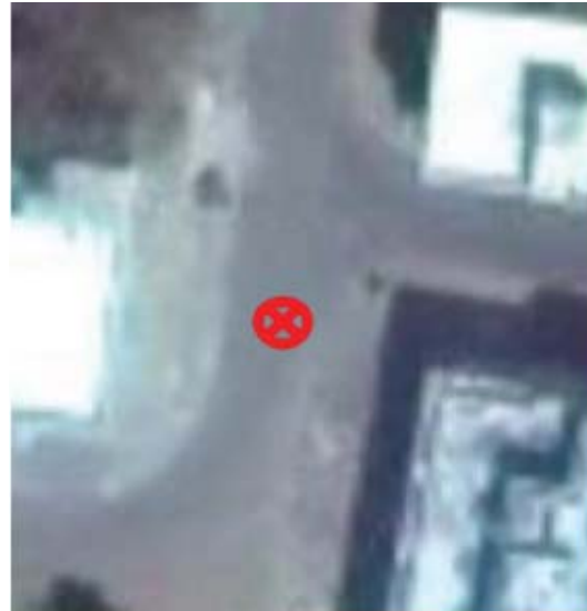
Figure 5: A single case input to CNN for estimating the class of the centre pixel
