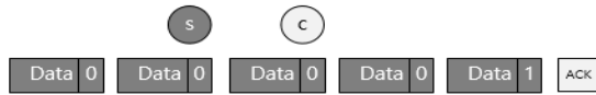
Figure 4: C Sends A Single ACK For Multiple Data Packet Received Independently From S
