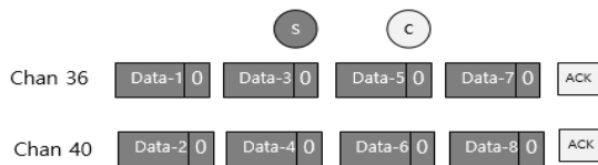
Figure 5: S sends 3 non-ACK packets on each channel and request for an ACK to acknowledge all packets on fourth packet on each channel.
