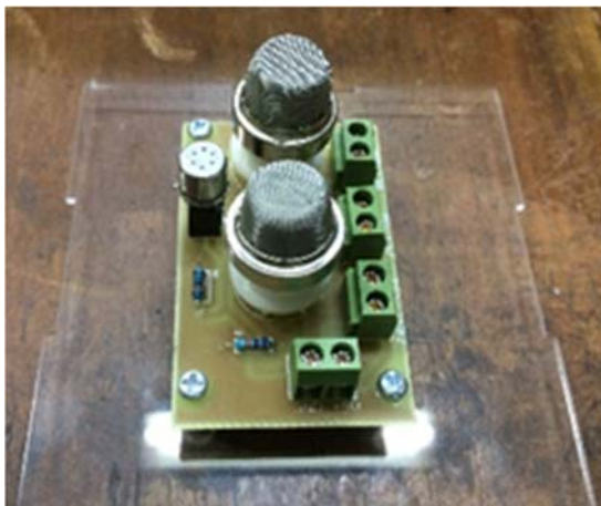
Figure 5: Placement of Gas Sensors in the designed PCB
