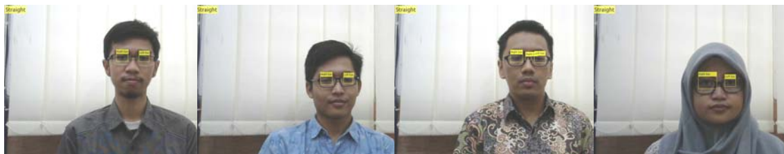
Figure 11: Samples of head movement detection of person with glasses based on Diagonal Coordinates Different (DCD)
