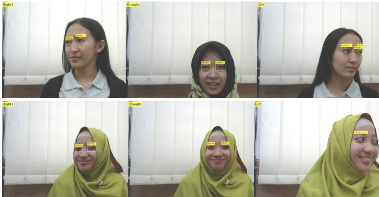
Figure 9: Result of head movement detection based on Diagonal Coordinates Distance (DCD)
