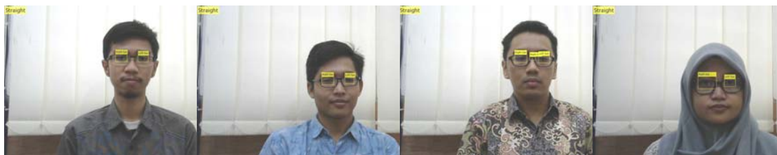
Figure 10: Samples of head movement detection of person with glasses based on Horizontal Coordinates Different (HCD)
