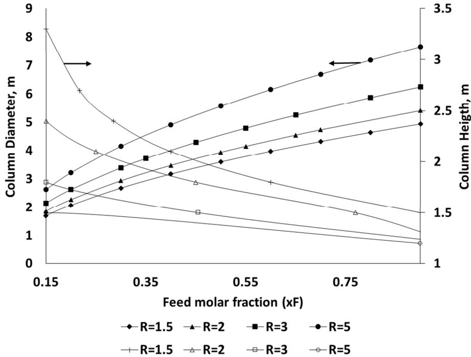
Figure 6. Effect of feed composition ( $x_F$ ) on column dimension ( $d, h$ ) under different reflux ratio ( $R$ ).
