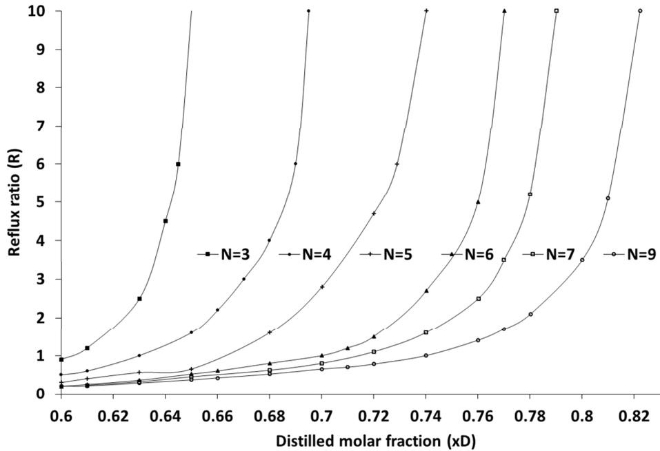
Figure 5. Effect of reflux ratio (R) on distilled molar fraction (XD) under different trays number
