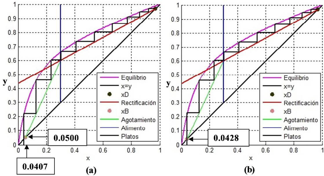
Figure 4. McCabe-Thiele operating line for rectifying and stripping section a) Composition with deviation of the real bottom molar fraction value b) Exact composition of the bottom molar fraction.
