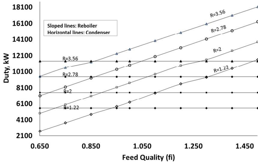
Figure 7. Effect of feed quality variation on condenser and reboiler duties under different reflux ratio
