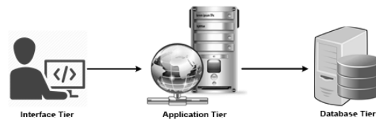
Figure 5 Tiers of the operational system architecture
