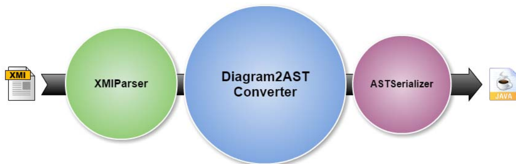
Figure 9: The Eclipse JDT-based code generator tool architecture.
