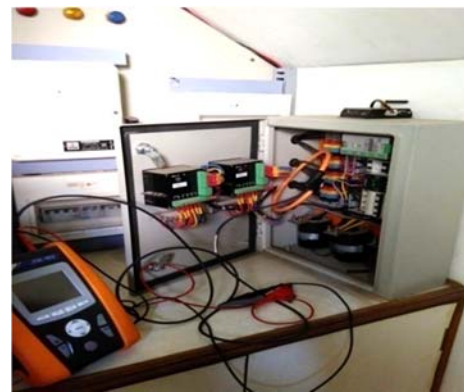
Figure 7 Internal Connection Of PQ Analyzer Connected To PV System
