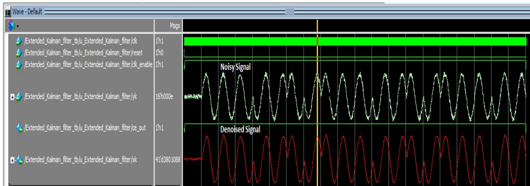
Figure 12: Proposed EKF method simulation result using Modelsim
