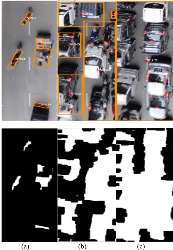
Figure 17. Road Density Reading Result: (1) Low-Density Condition; (b) Mid-Density Condition; (c) High-Density Condition
