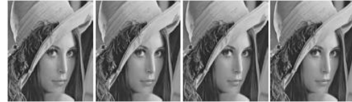
Figure 5: Part of Lena image with 200% magnification using 20% measurements. (a) Original image; (b) reconstruction using proposed E-NDLR with IST, PSNR=36:33dB; (c) TVAL3 + E-NDLR, PSNR=36:35dB (d) BCS-SPL + E-NDLR, PSNR=36:35dB. measurements. Also, we show in Fig. 5 the result of original E-NDLR using IST as well as TVAL3+E-NDLR and BCS-SPL+E-NDLR. They all have similar visual results as compared to the original image. This is consistent to the observation made based on Table 1 that their recovery PSNRs are very close.
