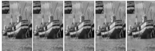
Figure 4: Boat image with cropped character patch using 20% measurements. (a) proposed E-NDLR recovery, PSNR=32:48dB; (b) NLCS recovery Shu et al. (2014), PSNR=30:66dB; (c) TVNLR recovery Zhang et al. (2013), PSNR=28:02dB; (d) NLR-CS recovery Dong et al. (2014a), PSNR=29:07dB; (e) NLTV recovery Zhang et al. (2010), PSNR=27:97dB.
