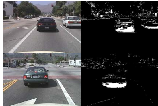
Fig.1. Vehicle detection based on shadow
