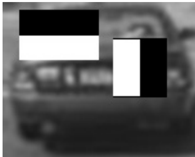
Fig.5. Extraction of haar features using the 2 rectangular filters (horizontal and vertical)
