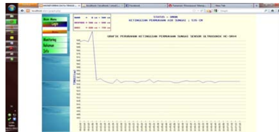
Figure 7: Real Time and On Line Graph of River Water Level Displayed on the Client Computer.
