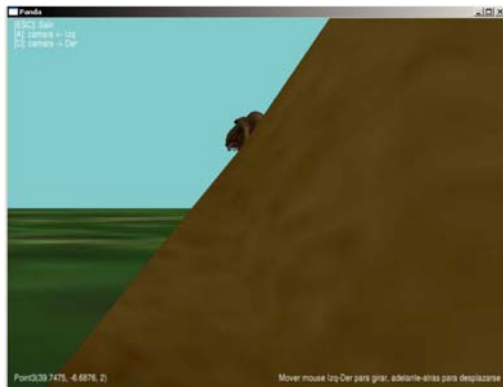
Figure 8. The Camera Is Unable To Traverse The Object (Rock) And Tends To Surround It.
