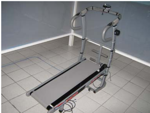
Figure 2. Treadmill Adapted As A Virtual Reality Navigation System.
