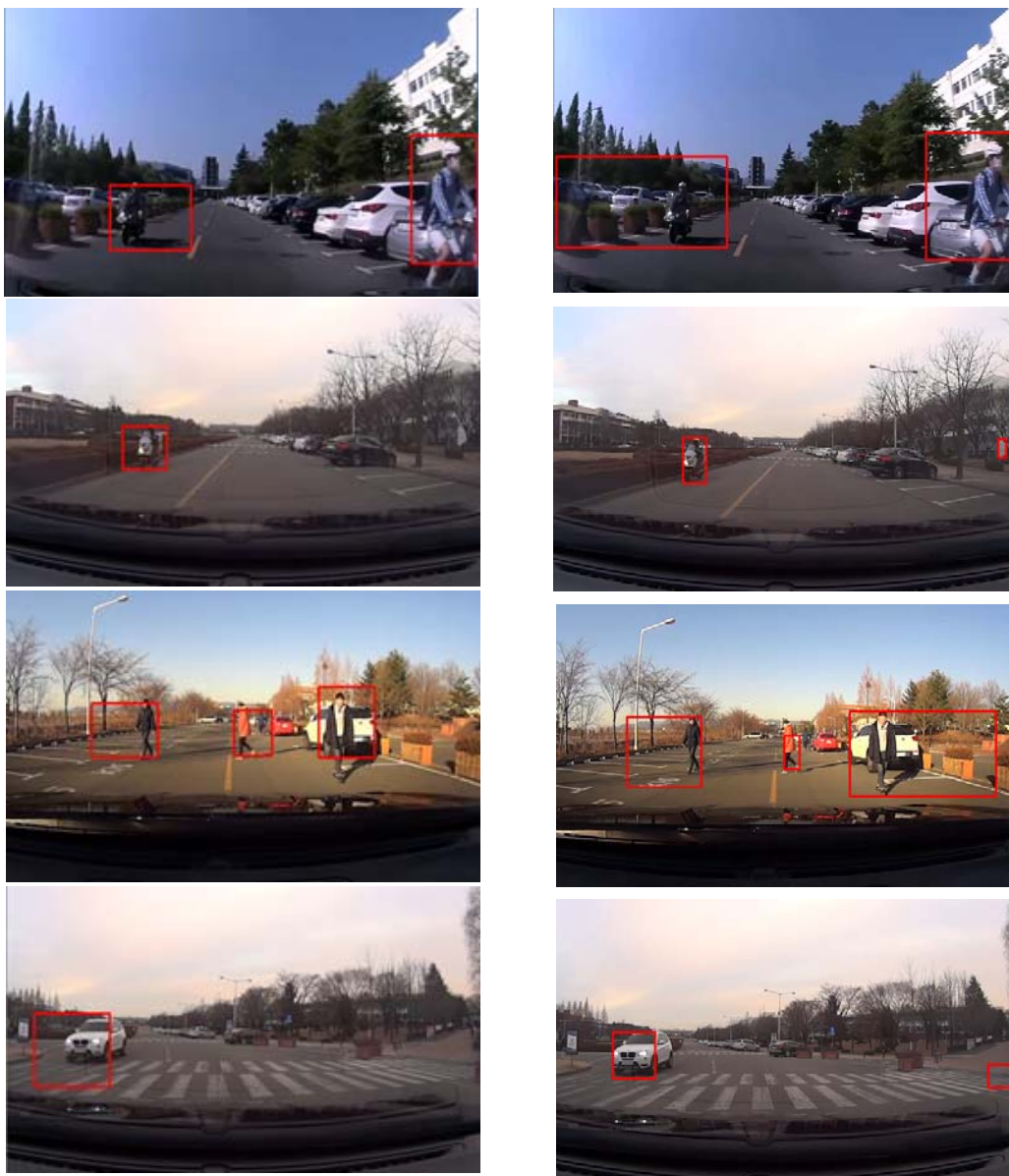
Figure 6: Examples of moving object detection of the proposed (left column) and Dual-mode SGM method[10] (right column) tested on dynamic scenes
