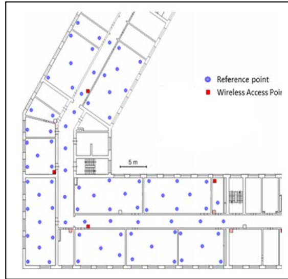
Figure 5: Layout Of The Testes Environment With Reference Points And Access Points
