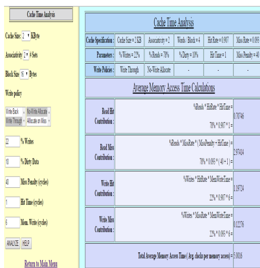
Figure. 13. Write Through - No Write Allocate
