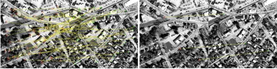
Figure 3: Matching point using BRISK with inliers and outliers, only with inliers
