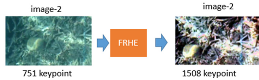
Figure 14. Keypoint detection results from FRHE method for image 2
