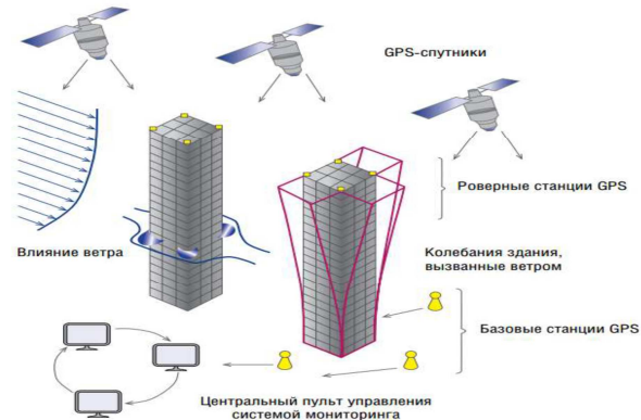
Figure 2 - GPS Monitoring Of Wind Impact On The High-Rise Building
