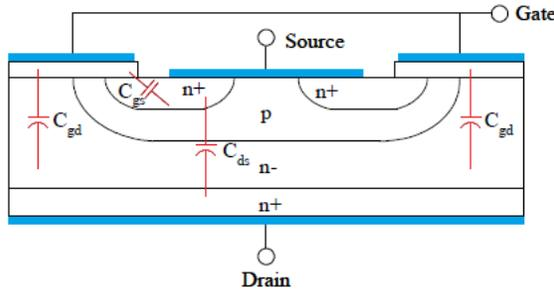
Figure 3 : Power MOSFET Structure Capacitances
