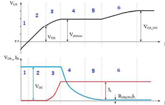
Figure 6. The current and voltage curves MOS turn-on phases
