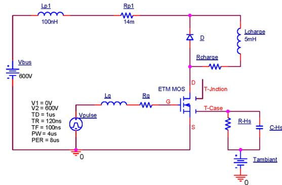
Figure.10: OrCAD Spice simulation schematic
