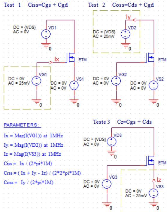
Figure.8: OrCAD Spice simulation circuits for MOSFET dynamic capacitances.
