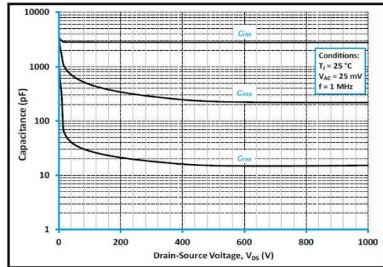
Figure 4 : Typical Capacitances vs  $V_{DS}$  (0-1000 V)
