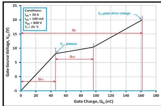
Figure 5. Typical Gate Charge Characteristic at 25°C
