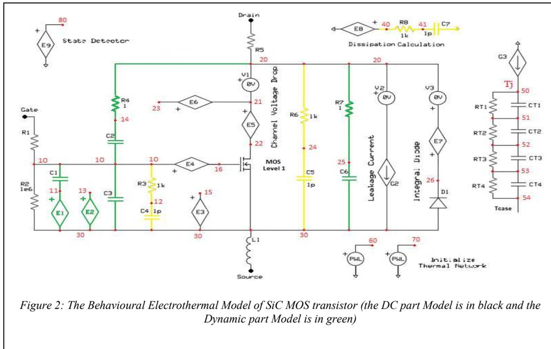
In switching the power SiC MOS acts as a power switch and the current  $I_D$  is controlled by the voltage  $V_{GS}$  (transfer characteristics). Its performance is defined by the time required to establish the voltage variations at the terminals of its physical capacitances within in the transistor which are composed of the gate oxide and the depletion layer as shown (Fig.3) [15].
