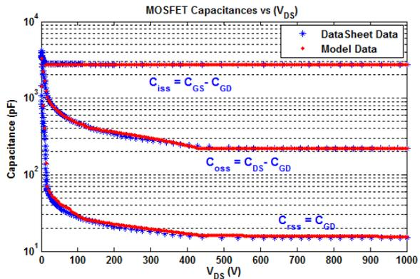
Figure.9: Curves of MOSFET dynamic capacitances  $C_{iss}$ ,  $C_{oss}$  and  $C_{rss}$ , vs  $V_{DS}$ .
