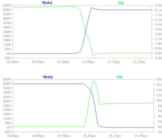
Figure 11. Voltage- Current Turn-off and Turn-on Switching Waveforms
