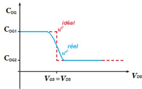
Figure 7. Capacitance  $C_{DG}$  variations vs  $V_{DS}$  Voltage (0-1000 V)
