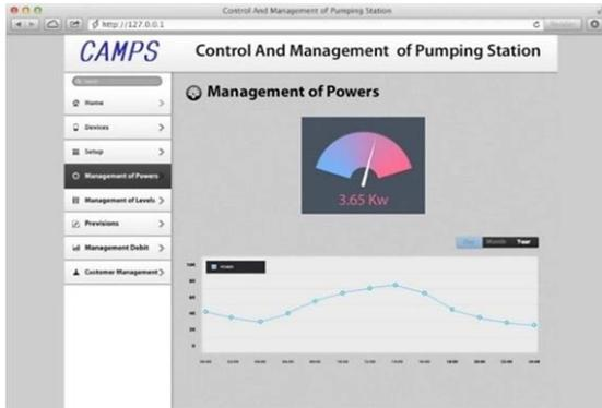
Figure 16: Web application screen in case of the powers management
