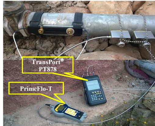
Figure 4: The flow meters PrimeFlo-T and Transport@PT878
