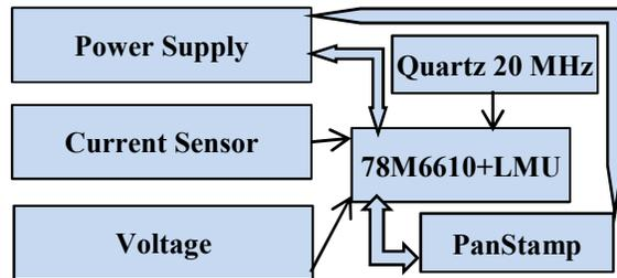
Figure 8: The power measurement block diagram
