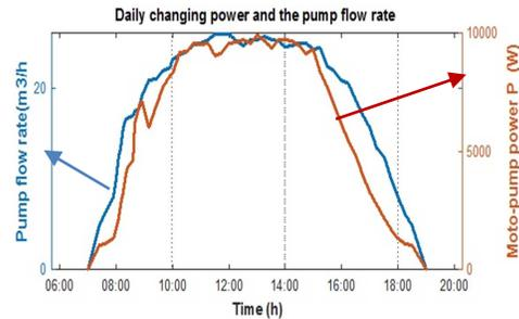
Figure 11: Evolution of Moto-pump power and the pump flow rate during May 27, 2016
