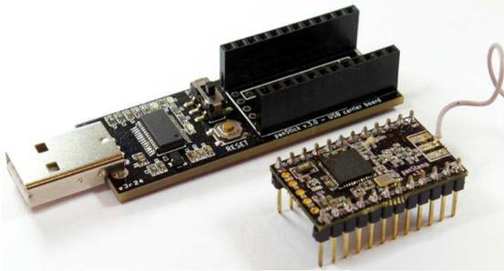
Figure 9: Module PanStamp at the bottom with its programming adapter
