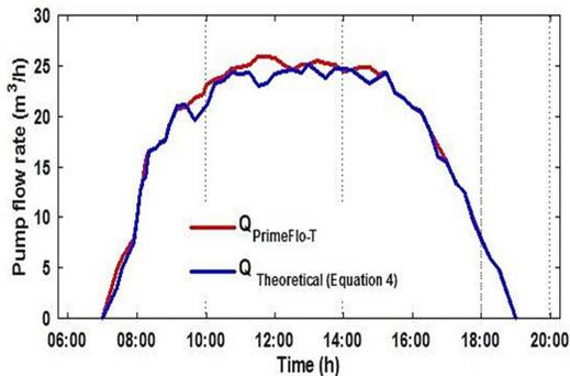
Figure 13: Comparison of measured and theoretical volumetric flow during 27/05/2016
