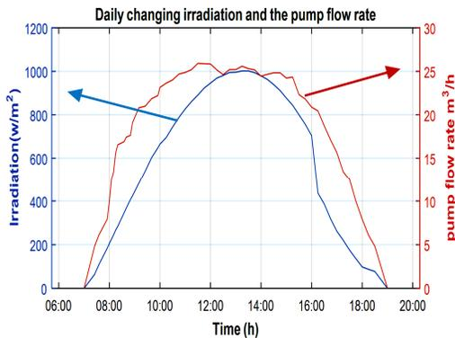
Figure 12. Evolution of the volumetric flow rate of the pump, measured with PrimeFlo-T and instantaneous radiation during May 27, 2016
