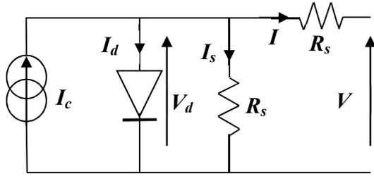
Figure 10: Equivalent to a single diode circuit [3]
