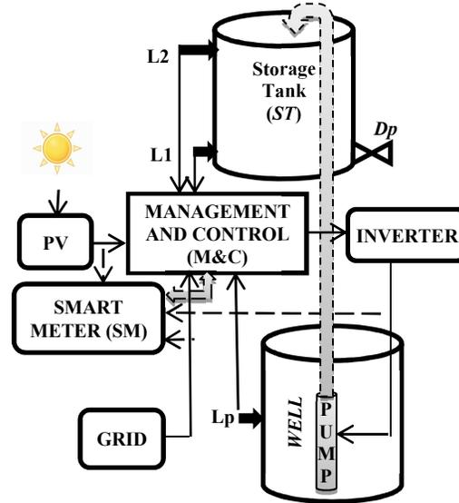
Figure 1: Description of the photovoltaic pumping station
