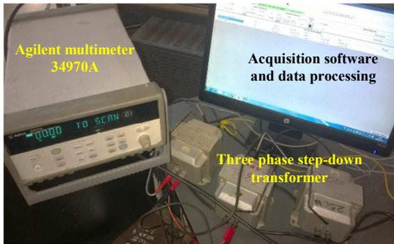
Figure 5: Agilent 34970A Data acquisition / Switch unit with its operating software and the three-phase step-down transformer
