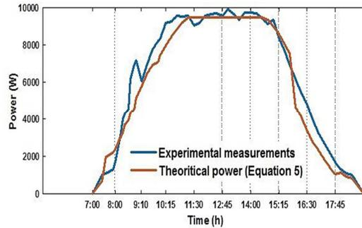
Figure 14: Comparison of the theoretical Moto-pump power P and measured powers during May 27, 2016
