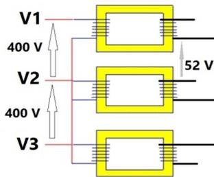
Figure 6: Wiring diagram of the three-phase step-down transformer with three single phase transformers
