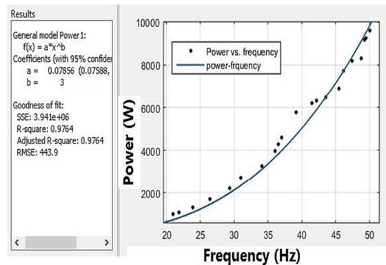
Figure 15: Relationship between power and frequency at the output of inverter
