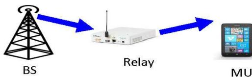
Figure 1: A downlink scenario in an AF relay network
