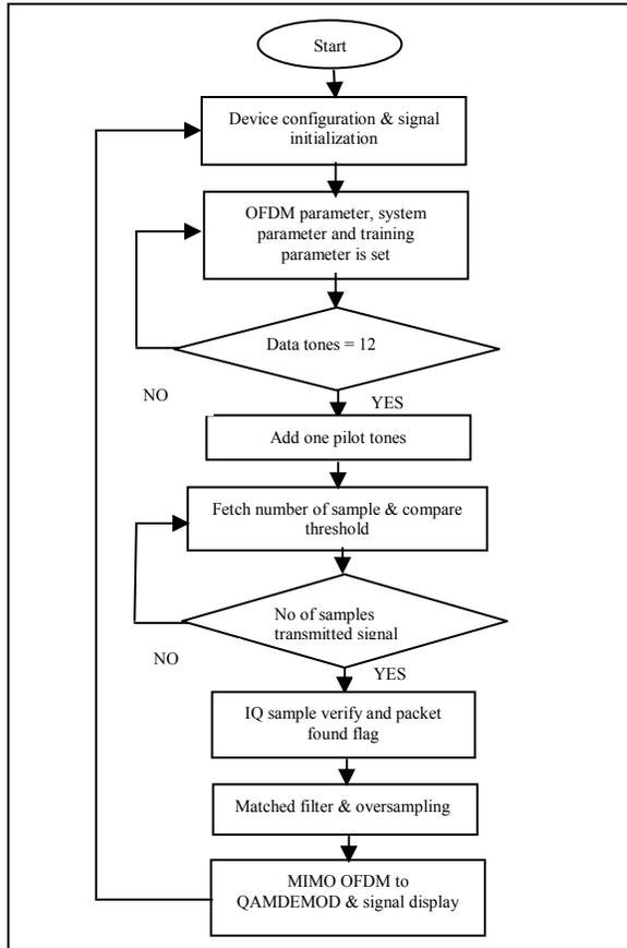
Figure 5 Flowchart of Destination Programming
