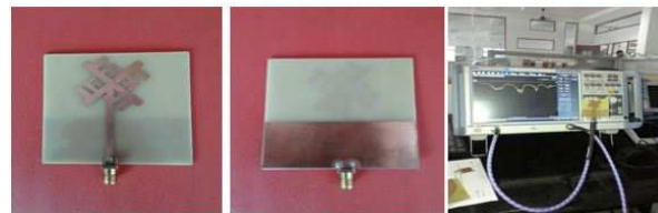
Fig. 15. Fabricated Antenna on FR4 Substrate and Testing on VNA
