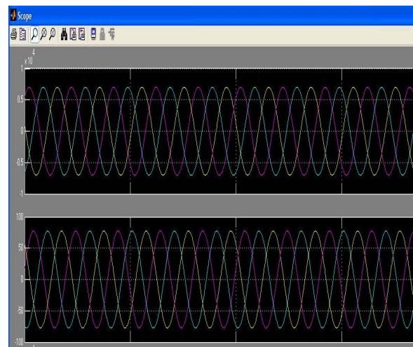
Fig 16 Compensated Voltage Signals at feeder 1 & 2 with IPQC
