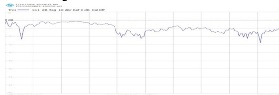
Fig 5.B Measured Return Loss For Model 2
