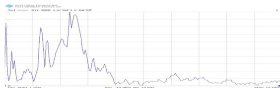
Fig 6.B Measured VSWR For Fabricated Antenna
