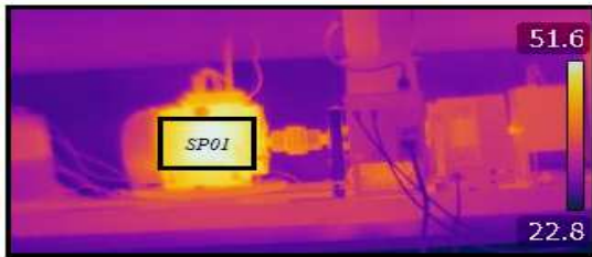
Figure.6. Thermal Image (Thermogram) With Correct Parameters, 60minutes Of Continues Operation With The Braking Torque [2.5Nm] Set In Camera FLIR T440. (See Table.9)
