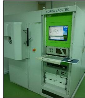
Figure 2: PVD Magnetron Sputtering Machine.
