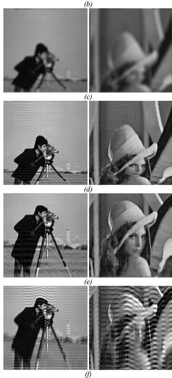
Figure.4 Restoration results of the conventional restoration algorithm and our algorithm (a)original image (b) defocus blurred image (c) space-invariant defocus image after nonlinear transform (d) the restored image of (c); (e) the restored image after nonlinear inversion transform from (d); (f) the restored image using conventional method from (a)
