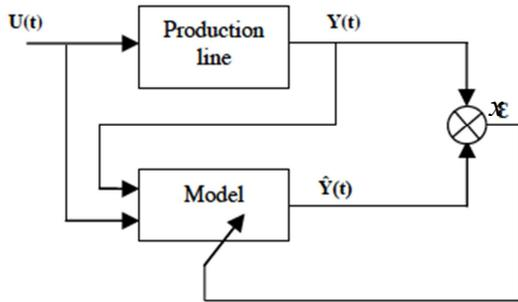
Fig. 2. Principle of identification based on the prediction error.
