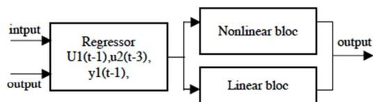
Fig.3. Structure of nonlinear autoregressive exogenous Model.
