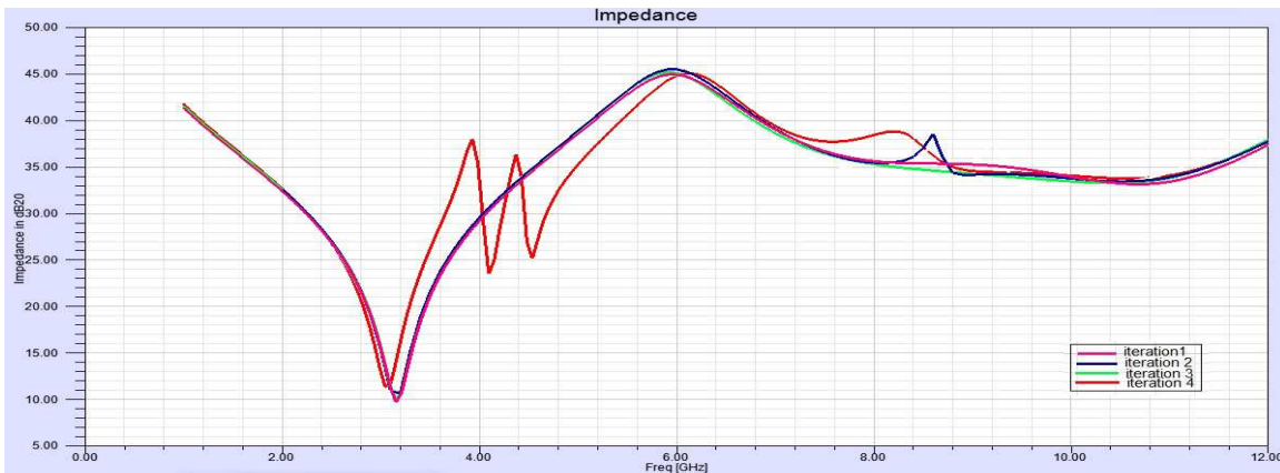
Figure 4 : Frequency Vs Impedance Of Different Iterations
