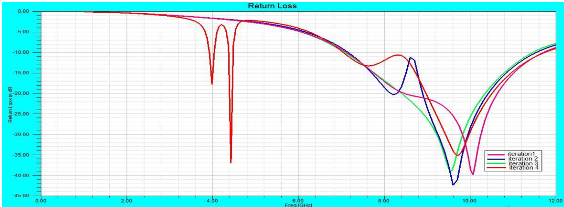
Figure 3 : Frequency Vs Return Loss Curve For Different Iterations
