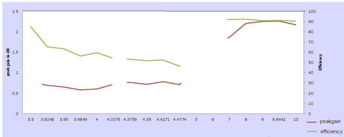
Figure 14 : Frequency Vs Gain And Efficiency Of The Proposed Antenna
