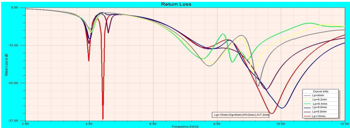
Figure 6 : Parametric Analysis With Change In L_p
