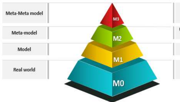
Fig 5: MDA 4 Levels Architecture
