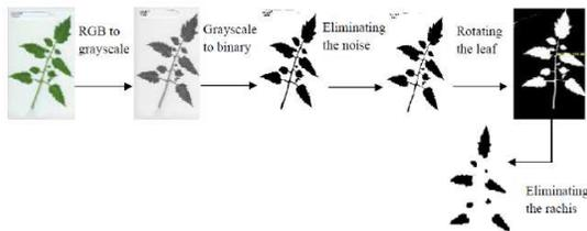
Figure 2. An Image Of A Tomato Compound Leaf In The Pre-Processing Stages.
