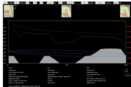
Figure 9: Profile Terrain From BWA Station Towards FSS ES (Point 18)
