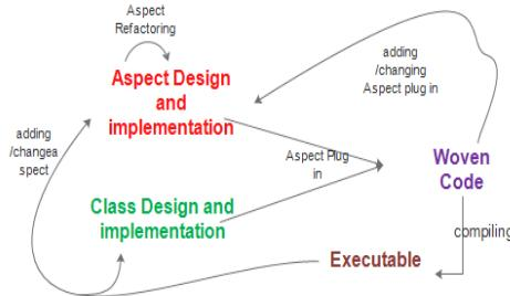
Fig. 2 (Process Of Aspect-Oriented Development Stages)
