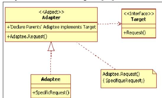
*Fig. 11 (Adapter Pattern In Aspect Class Diagram)*
