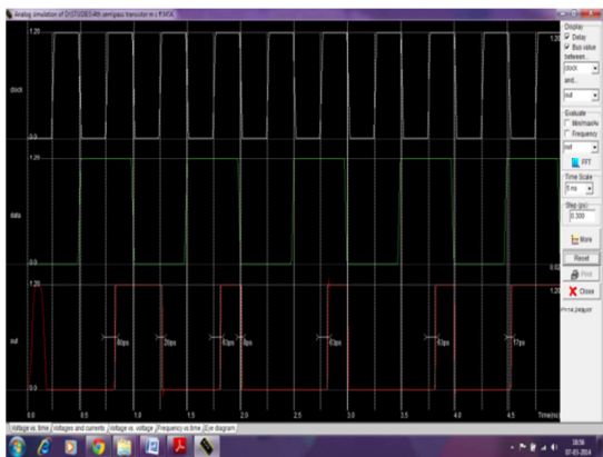
Figure11: Output Waves For Master Slave Flip Flop By Using Pass Transistor
