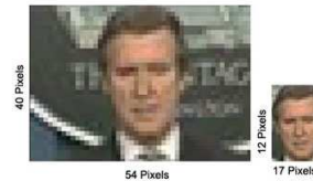
Figure 12: Sample Of Face Detection In Image With Low Resolution Of 54 ×40 Taken From Caltech 10000 Database.
