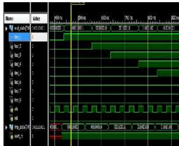
Figure 8: Uart Receiver Results
