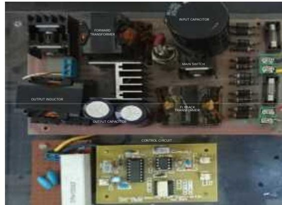
Figure 16. A Prototype Of The Proposed Dc Power Supply With Power Factor Correction
