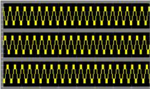
Figure 16. Line Voltage For Three-Level Inverter At MI= 0.8.
