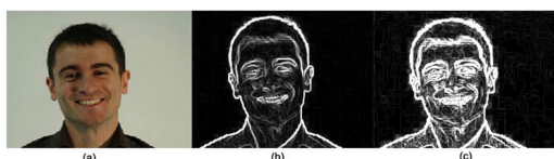
Figure 10: Edge Detection Result (a) Original Image (b) Detected edges by Sobel 3x3 (c) Detected edges by Kirsch.
