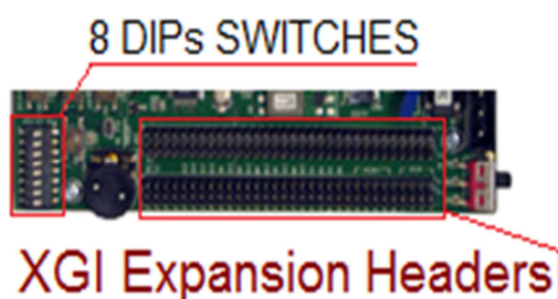
Figure 5: Extensions Connectors (XGI) and 8 Dips Switches.
