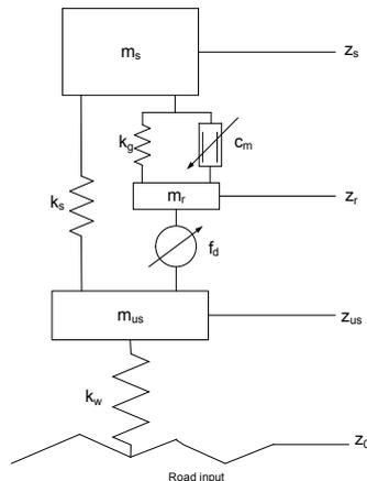
Figure 7: Quarter Car Model with Electromagnetic Damper
