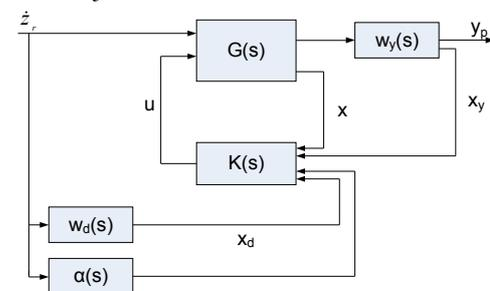
Figure10. Multi objective  $H_\infty$  control scheme
