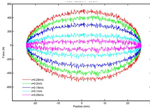
Figure 5. Force-distance diagram for different velocities,  $R=20ohm$
