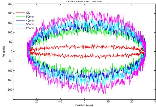
Figure 4. Force-distance diagram for different electrical loads with  $v=0.2m/s$
