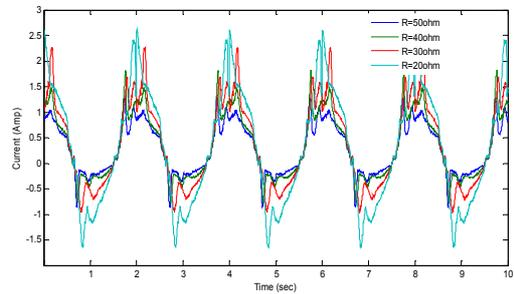
Figure 6. Generated current,  $v=0.2m/s$  for different electrical loads.
