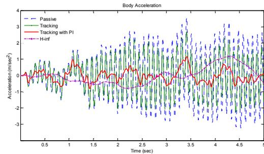
Figure 13. Sprung-mass body acceleration
