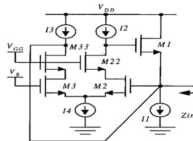
Figure 5 Double Feedback With Second Order Circuits[3]
