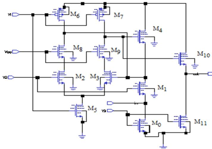
Figure 6 Schematic Of Proposed Low Noise Amplifier[3]
