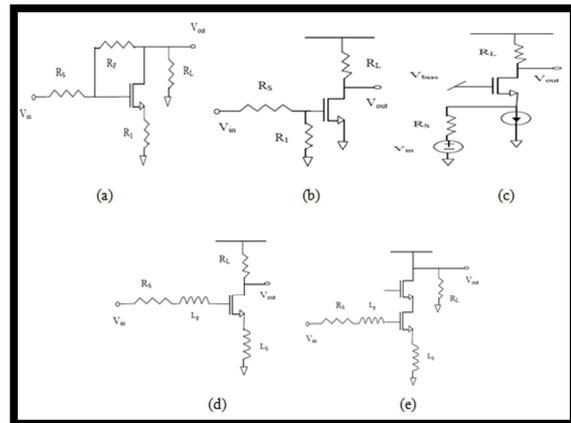
Figure 2 Fundamental Of Topologies LNA: (A) Shunt Series Feedback Common Source (B) Inductive Degeneration Common Source (C) Common Gate (D) Resistive Termination Common Source (E) Cascade Inductor Source Degeneration[2]
