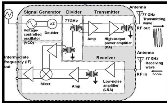
Figure 1 Block Diagram Of RF Transceiver[1]
