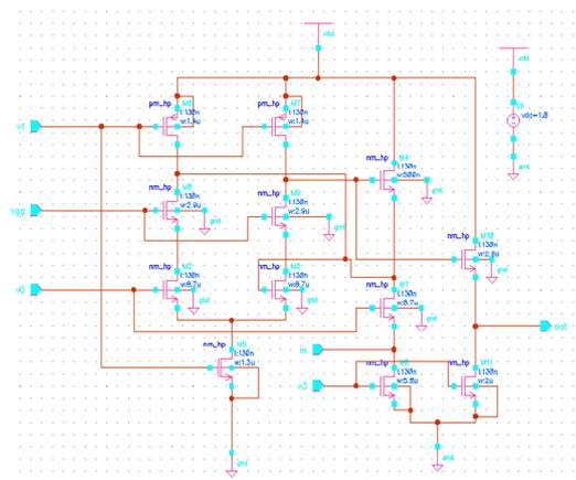
Figure 7 Schematic Of Proposed Low Noise Amplifier After Enhancement
